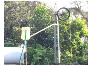
10. Rope and Washer Pump: Monsoon Farm
